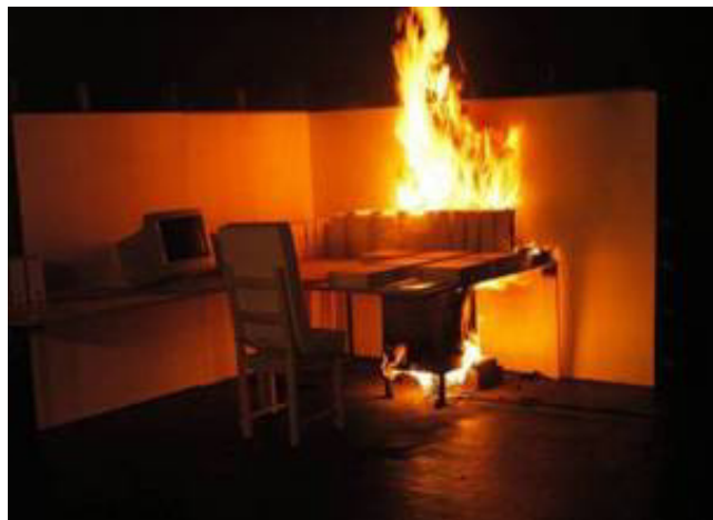
Fig. 8: Fire test according to CEN/TS 14972, OH1 Office
